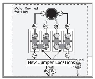
Figure 5. Relocated jumpers.
